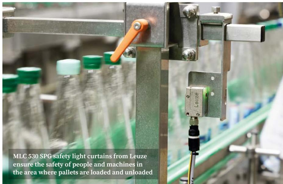
MLC 530 SPG safety light curtains from Leuze ensure the safety of people and machines in the area where pallets are loaded and unloaded
