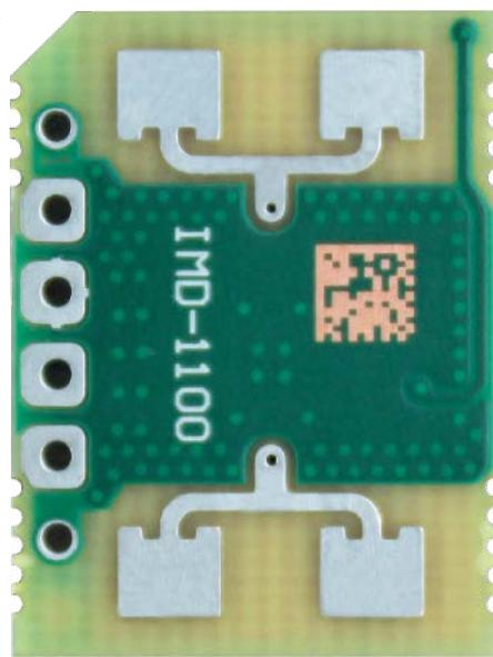
**The latest addition to Innosent's radar range: The IMD-1100 radar, the smallest 24 GHz radar available in their portfolio**
