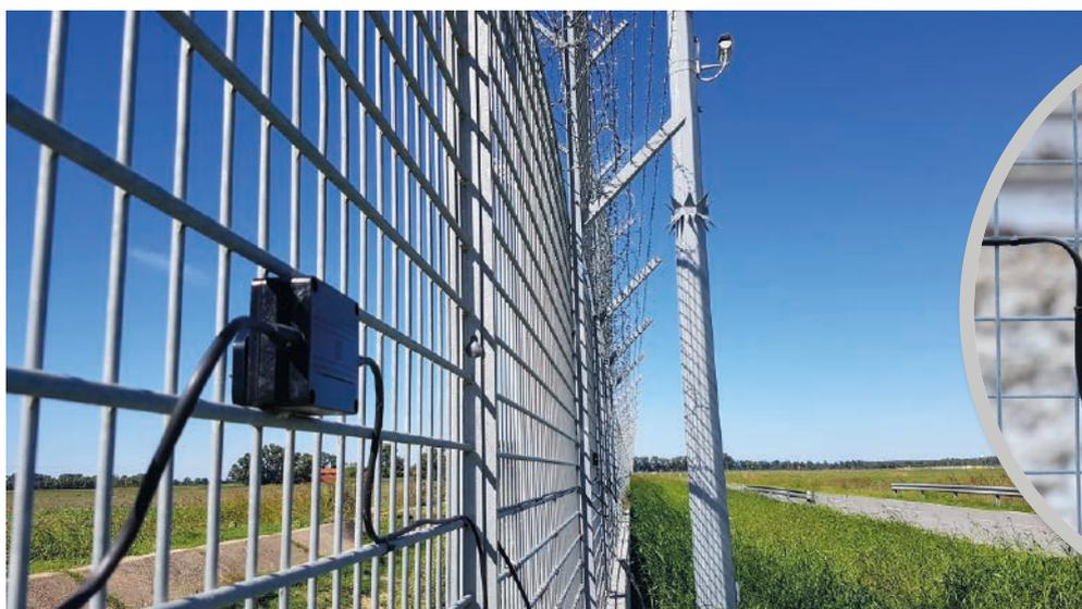
Detection of any climbing, cutting, lifting the fence or displacing of the sensors
