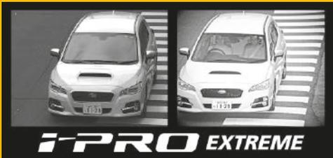
The camera comes with a multiple shutter mechanism and a resolution of 5 MP in connection with outstanding camera features (wide dynamic range, outstanding light sensitivity). All those parameters make the recording of moving vehicles including number plates and the face of the driver at the same time possible.
