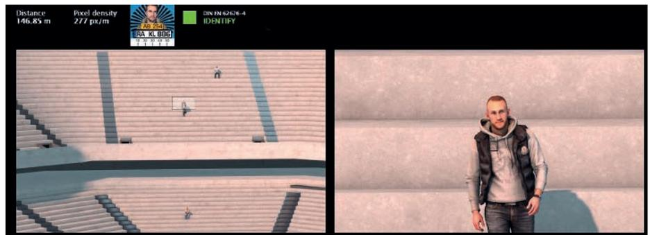
**Specifying the required pixel density for the job at hand during the planning phase ensures that the best possible images are obtained**
