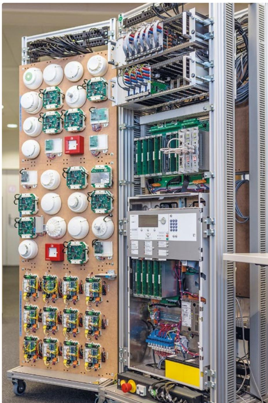
An automated test system is a combination of real and simulated components ►
