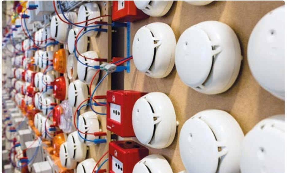
The test system can simulate all kinds of situations and perform a virtual compliance check
