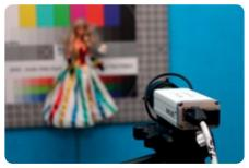
Rotating doll: the test conditions in the SeeTec Competence Center, where the GIT SECURITY camera tests are performed, are the same for all cameras
