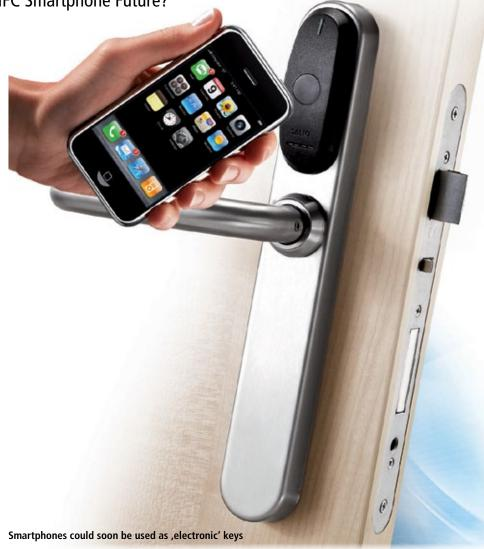
popular consumer level wireless technologies. The main difference between RFID and NFC is that while RFID can be used beyond a distance of a few metres, NFC has a very small range and is used where a more secure method is needed, such as using a contactless credit card to pay for something or unlocking a door. In essence, NFC is an extension of RFID, but it is more secure.
