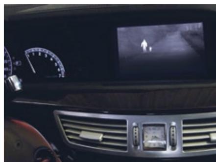
The thermal images generated by the PathFindIR can be displayed on any multi-function LCD display that accepts composite video. In this case on an LCD integrated in the Mercedes dashboard.
