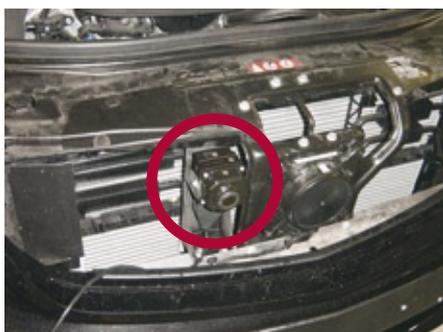
The FLIR Systems PathFindIR installed behind the vehicle grid of an armored Mercedes.
